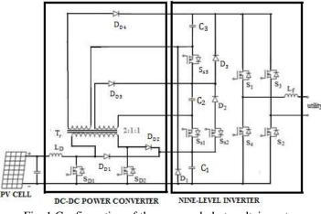
Fig .1.Configuration of the proposed photovoltaic system
