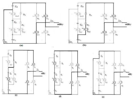
Fig.4. Operation of the nine-level inverter in the negative half cycle (a)mode 6,(b) mode 7, (c) mode 8, (d) mode 9 and (e) mode10.
